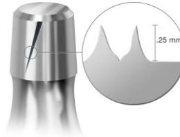
Taper with scratch/defect at a Height of 0.25mm – Figure A
