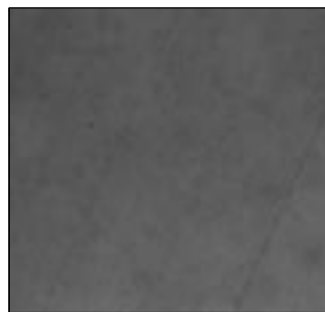
100x Magnification—Cross-section of an ArCom isostatic uniform molded acetabular liner showing highly consolidated material.
