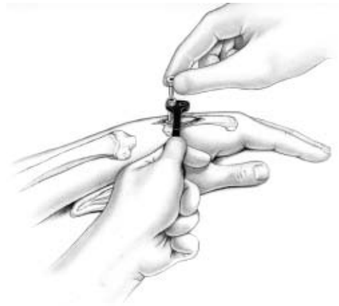
Insert appropriate drill guide into bone screw template.
