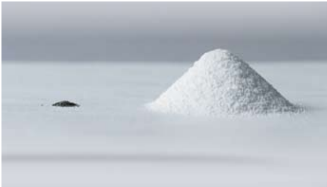
Figure 1: Representative of 25 years cumulative metal-on-metal wear debris vs. 25 years cumulative polyethylene wear debris. 1,4
