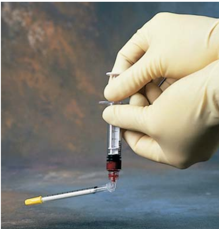
Figure 2. Attach the hydrating fluid of choice by twisting the syringe on to the Luer Lock fitting. NOTE – in all subsequent steps, the syringe with hydrating fluid must be pointing down as illustrated.
